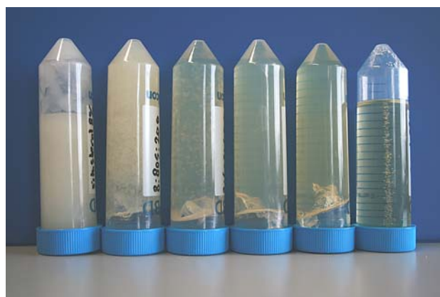
Fig. 3 Mixtures of 8% \beta -sitosterol + \gamma -oryzanol in sunflower oil in various sterol(ester) ratios. The \beta -sitosterol: \gamma -oryzanol ratio from left to right: 100:0; 80:20; 60:40; 40:60; 20:80; 0:100. Both single sterol(ester) systems in sunflower oil are liquid, the binary sterol(ester) systems in sunflower oil are gelled. The firm gelled samples were scooped near to the cap, leaving a distinct fracture pattern
